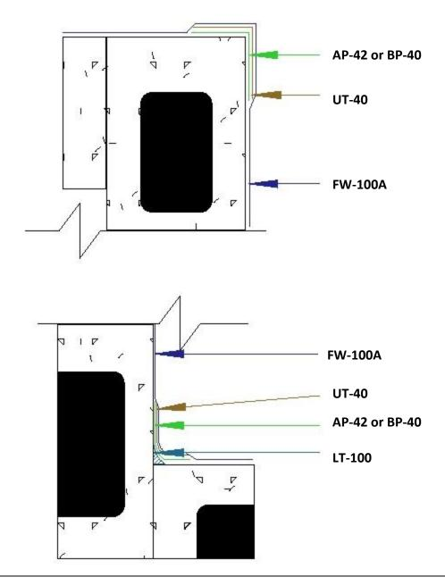
**Notes:** The AP-42/BP-40 and UT-40 may be replaced with an additional application of FW-100A, applied at 40 wet mils extended 3"'s past the corner on each side. This should total the coverage rate of FW-100A to a wet film thickness of 80 wet mils. All applications must be applied such that a void and pinhole free surface is achieved.
